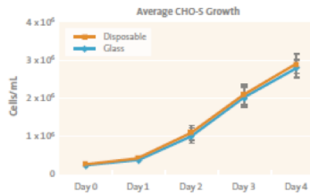
Figure 1: 96 hour growth of CHO-S cells in glass and disposable 1L spinner flasks from 3 studies at 60 rpm (n = 6). \pm S.E. indicated by error bars; p < 0.05 .
