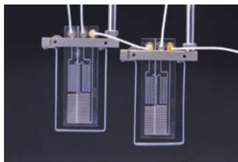
Figure 20: Two-stage assembly of two Sigma-Aldrich glass microreactors
