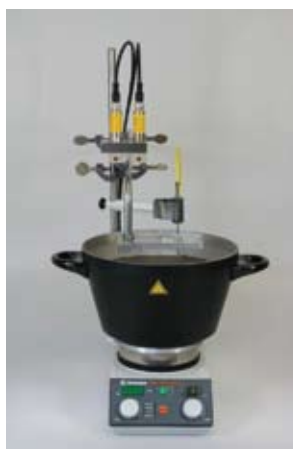
Figure 14: Set-up example with heated bath (not included in kit)
