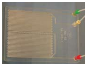
Figure 9: Two-layered XXL-version (15 mL) of Sigma-Aldrich's glass-microreactor manufactured by Little Things Factory
